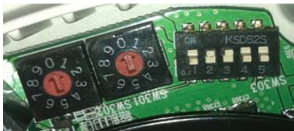
Figure 6.3 Close-up of Rotary Switches and Dip Switches
